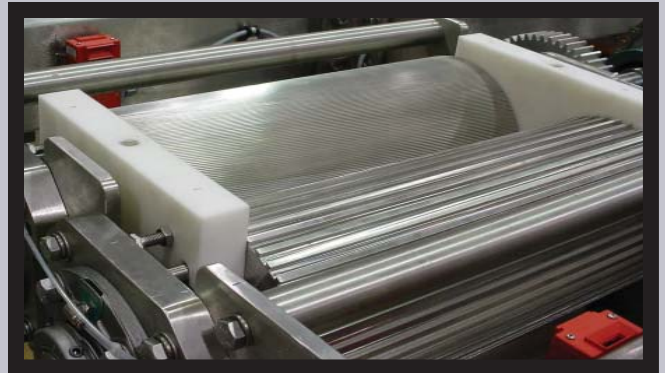
Upper Rollers Beneath Hopper
